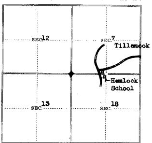
Information needed to find corner again: Cor. Consists of 4 big rocks in a pile 24" high. Metal loc. poster is on a BH tree 20" on the N side of tree from maich this cor. bears N 12".
